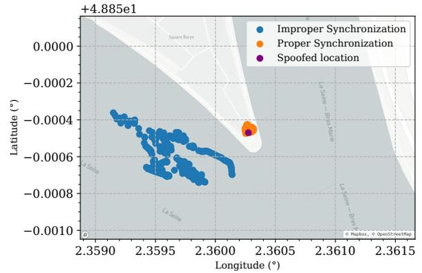
Figure 14: **Effect of GPSDO alignment.** Synchronization amongst transmitters depends on the stability of GPSDO. When clocks are synchronized (orange trace), the spoofed location is very close to the target location with an average error of only 2.0768 m. In contrast, unsynchronized clocks (blue trace) result in a larger average error of 48.9977 m.
