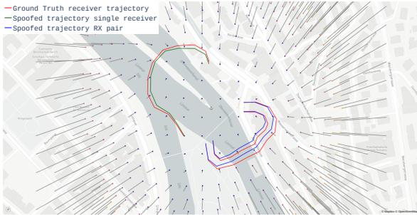
Figure 16: **Trajectories.** Under spoofing, trajectories closely match the ground truth. The attack bias does not significantly distort the acceleration/direction, like for relative distances. Hence, GPS data would be consistent with noisy INS data. Spoofing signal change naturally with the victim’s position relative to the transmitters, without attacker’s intervention.
