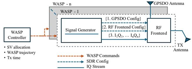
Figure 6: **Design Schematic** A WASP controller performs satellite allotment and sends a common transmission to WASP units. Each WASP unit is responsible for shadowing and impersonating a single satellite.
