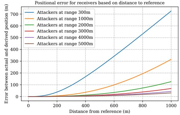
Figure 5: **Position error magnitude** estimated with the model. Curves are small and flat near the reference location (attack area), then start turning (border), and finally grow linearly (outside area). Greater satellite distance increases coverage.
